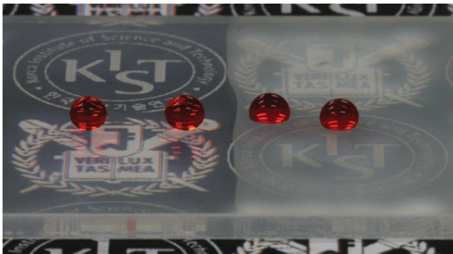
Figure 3. An optical image of one CF 4 plasma-treated and hydrophobic-coated sample on which the left half underwent the hydrolysis process and shows more transparency and hydrophobicity than the right half, which was completed without the hydrolysis process.
